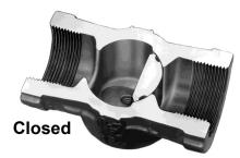
In the closed position, the plug makes contact with the seat. The resilient plug seal is pressed firmly into the seat for dead-tight shutoff. Eccentric plug and seat design assure lasting shutoff because the plug continues to move into the seat until firm contact and seal is made.
