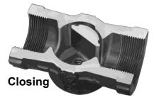
As the plug closes, it moves toward the seat without scraping the seat or body walls so there is no plug binding or wear. Flow is still straight through making the throttling characteristic of this valve ideal
