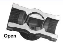
**KEY PORT** eccentric action and resilient seating assure lasting dead-tight shutoff. As the eccentric plug rotates 90 degrees from open to closed, it moves into a raised eccentric seat.
