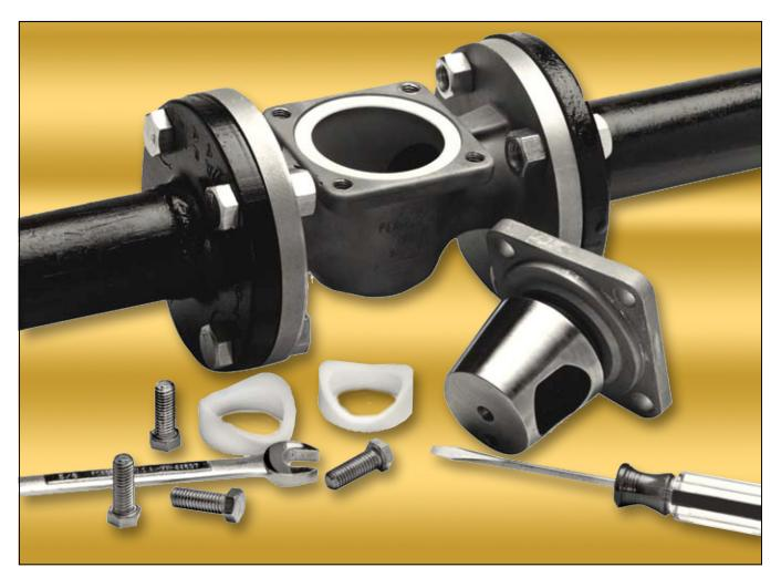
The Permaseal<sup>®</sup> valve's unique top entry design allows seat replacement without removing the valve from the line. Using only a wrench and screwdriver, worn seats are removed and new seats inserted in as little as 10 minutes.
