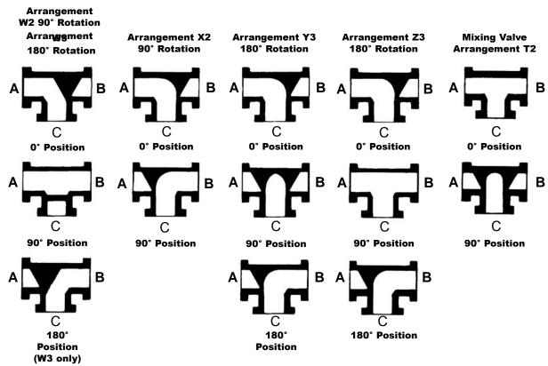
**Note:** Three-way plugs are recommended for diverting applications, with pressure at port C. Mixing applications with pressure at ports A and B may result in leakage.
